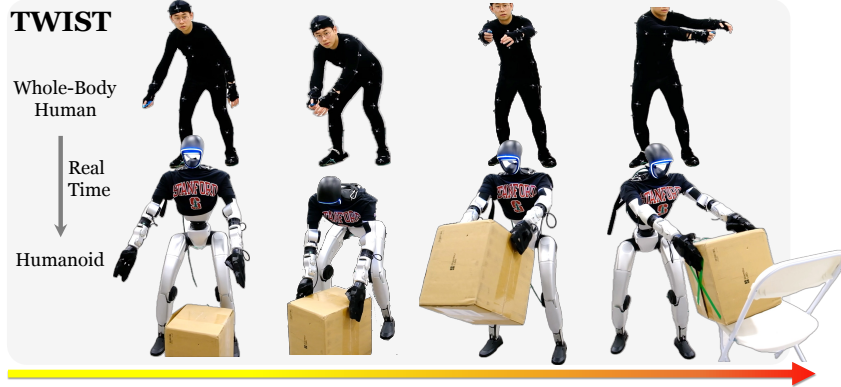
Figure 1: The Teleoperated Whole-Body Imitation System (TWIST) is a system that teleoperates humanoid robots with real-time whole-body human data and a single neural network controller. TWIST achieves versatile, coordinated, whole-body skills that are not present in previous works.
