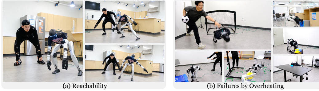
Figure 9: (a) Extreme reachability by TWIST. (b) Failures caused by motor overheating.
