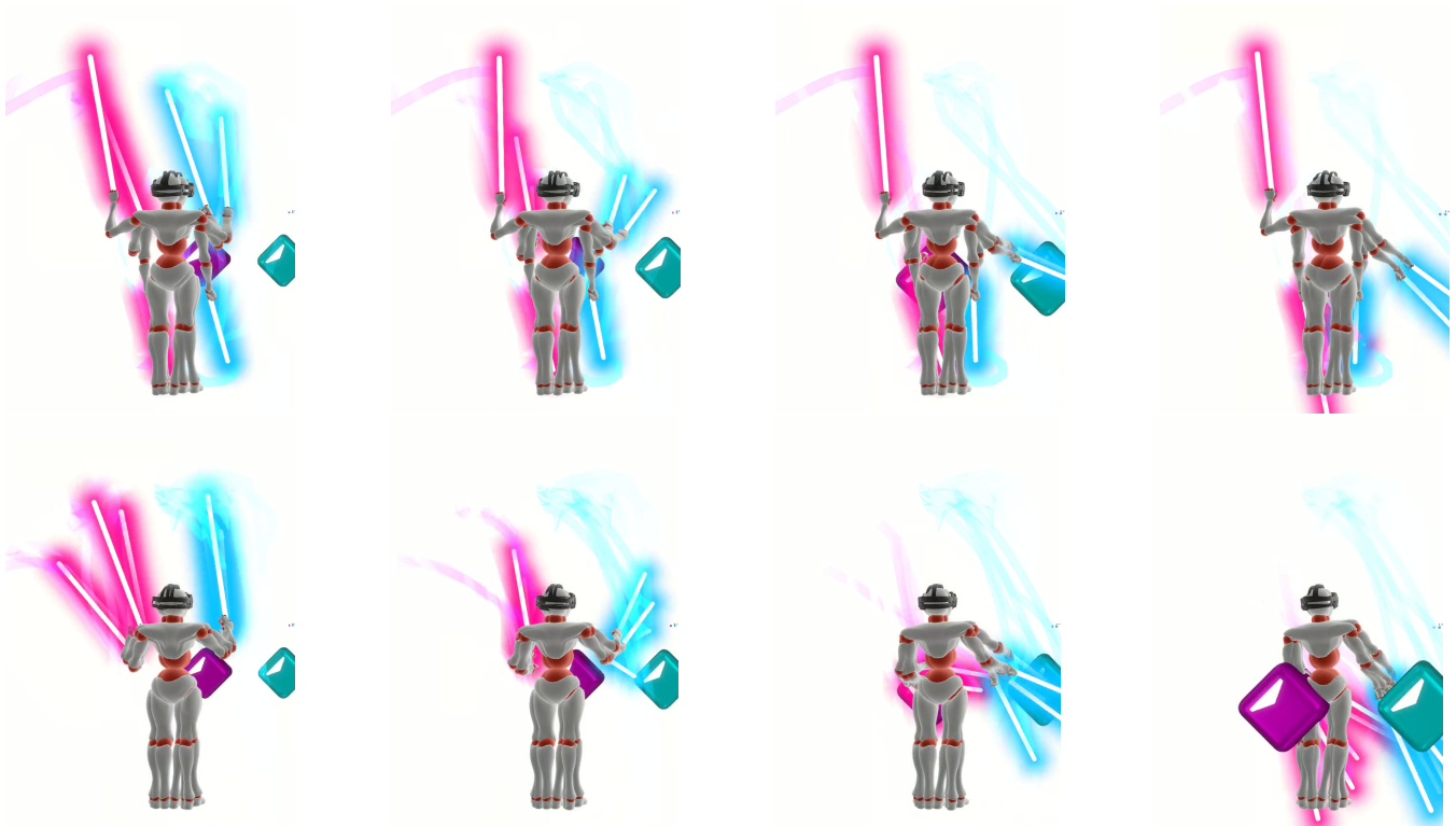
Figure 14: Top: Conditioning Robo-Saber on different \mathbf{x}^{N_{ref}} induces variations in behavior. Some correct and incorrect saber movements emerge, reflecting skill level variations present in conditioning signals. Bottom: Varying the random seed instead while conditioned on the same reference, the movement variation is less noticeable.
