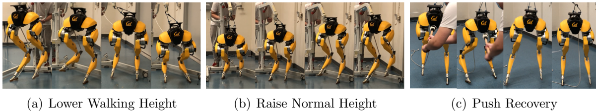
Figure 9.1: Our system is able to learn robust parameterized locomotion controllers for a bipedal Cassie robot. The controller can vary parameters such as walking velocity and height, while also being robust to significant external perturbations. (Video 1 )
