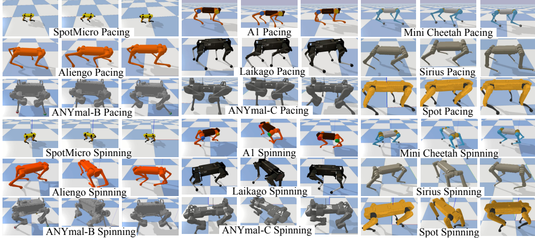
Figure 4: GenLoco policies deployed on a collection of quadrupedal robots that exist in real life. Two separate models are trained to perform a pacing gait and a spinning gait respectively. The GenLoco policies are trained in simulation using only procedurally generated robots, and robots used for testing are not used in the training process. The learned controllers can be directly deployed on all of these robots, including the ANYmal-series robots which have a distinct knee joint design, to perform agile maneuvers without additional training.
