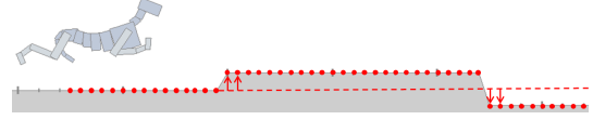
Figure 6: Terrain features consist of height samples of the terrain in front of the character, evenly spaced 5cm apart. All heights are expressed relative to the height of the ground immediately under the root of the character.
