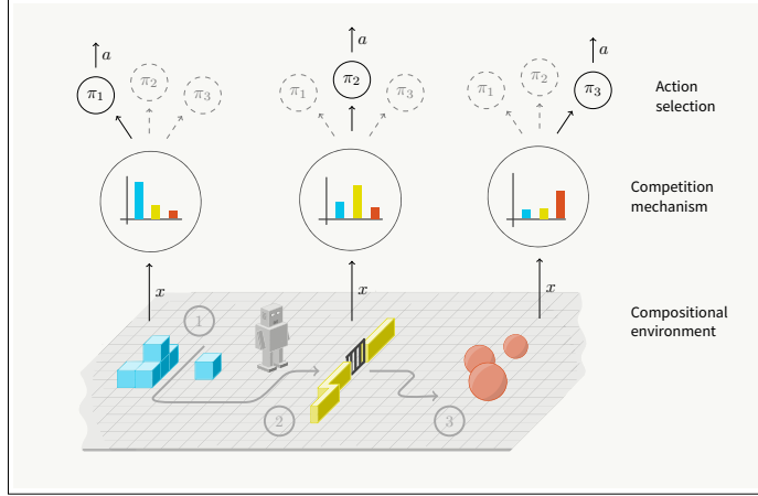
Figure 1: Illustration of our model. An intrinsic competition mechanism, based on the amount of information each primitive provides, is used to select a primitive to be active for a given input. Each primitive focuses on distinct features of the environment; in this case, one policy focuses on boxes, a second one on gates, and the third one on spheres.
