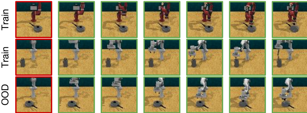
Figure 7: Sampled video predictions for in distribution reference videos (Train) and an OOD arm/task combination (OOD). The video model displays cross-embodiment generalization to arm/task combination not observed in the training data. Video model generalization can enable specifying new tasks where no reference data is available.
